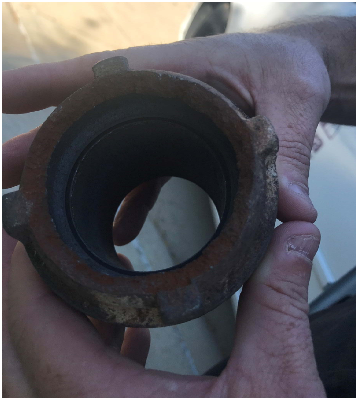
Figure 3: The failed cap after it had been removed from the steam pipe.
