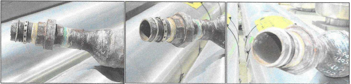
Figure 17: A coupling and fractured section of piping was located at the end of the section for in-line valve and regulator.
