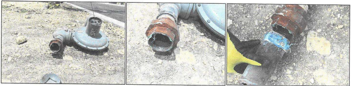
Figure 19: The coupling on regulated side of natural gas line matched a section of pipe found in the courtyard/loading dock area.
