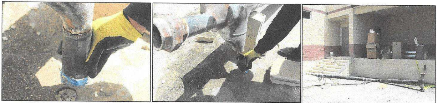
Figure 20: A large section of natural gas line was located next to the loading dock and was identified as the "tee" which split gas supply between the boilers and the water heaters. The section of pipe from Figure 19 matches the weld of the "tee."
