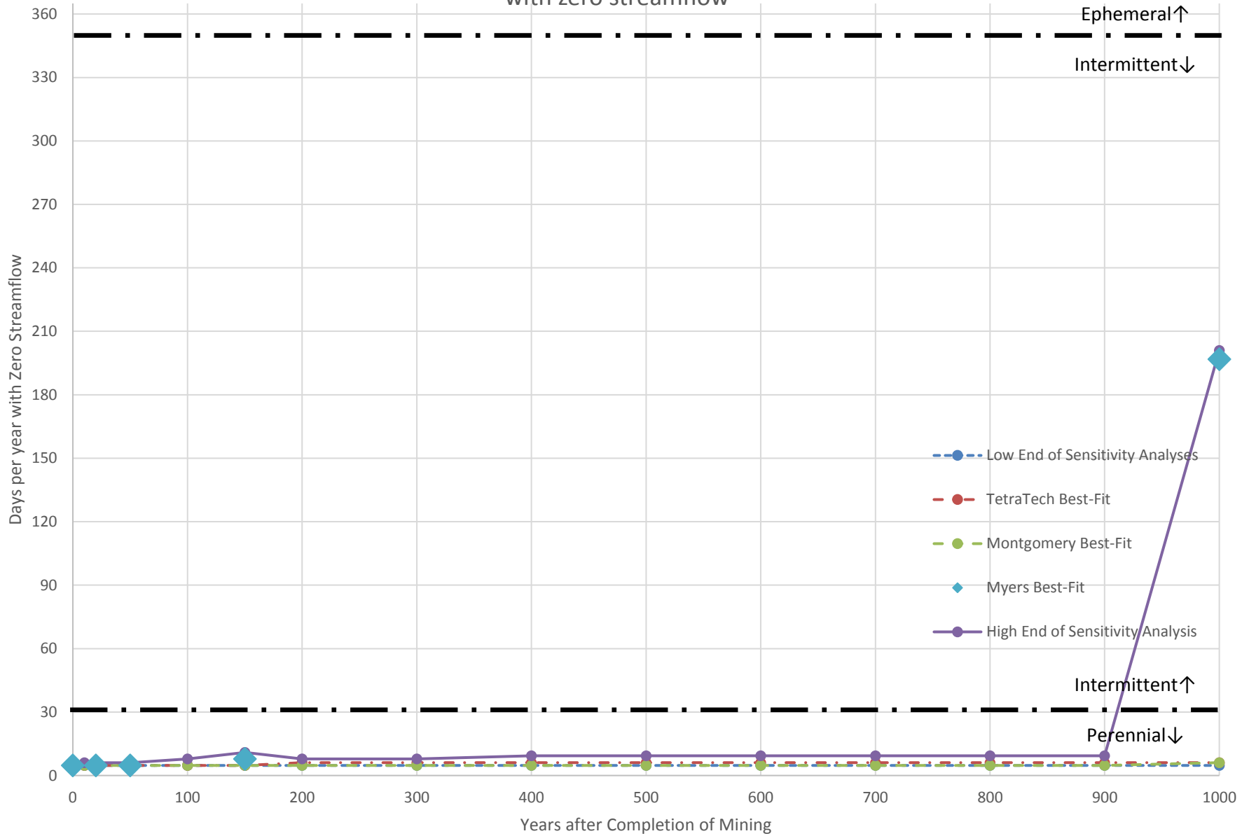
Figure H3-B1. Refined streamflow prediction, CC5, Combined Mine and Climate Change, Days with zero streamflow
