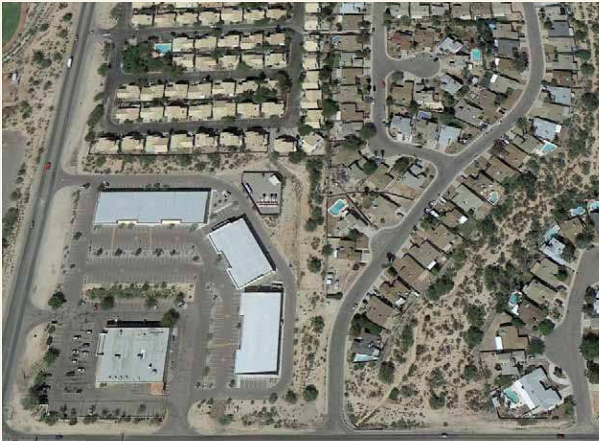
Low street connectivity makes it inconvenient for residents to walk to commercial services.
