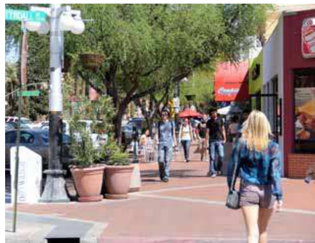
Pedestrian-oriented street near the University of Arizona. The clearly defined sidewalk zone system, wide clear area, shade trees, on-street parking and structures built to the sidewalk contribute to a high-quality pedestrian experience.
