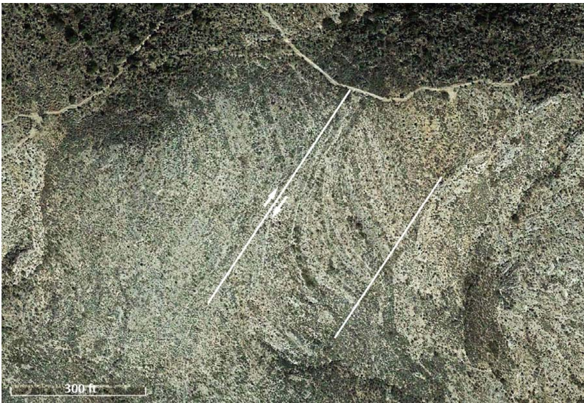
Figure 2. Drag folds along an oblique-slip or strike-slip fault in the Paleozoic Escabrosa Limestone on the hill north of the caverns demonstrating right-lateral displacement. A second parallel fault is marked that truncates beds. This exemplifies the intense deformation of the Kartchner block.
