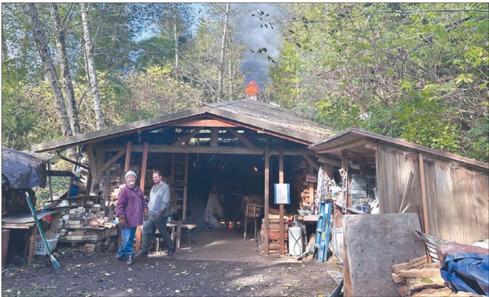
The Anagama kiln during the firing process.
