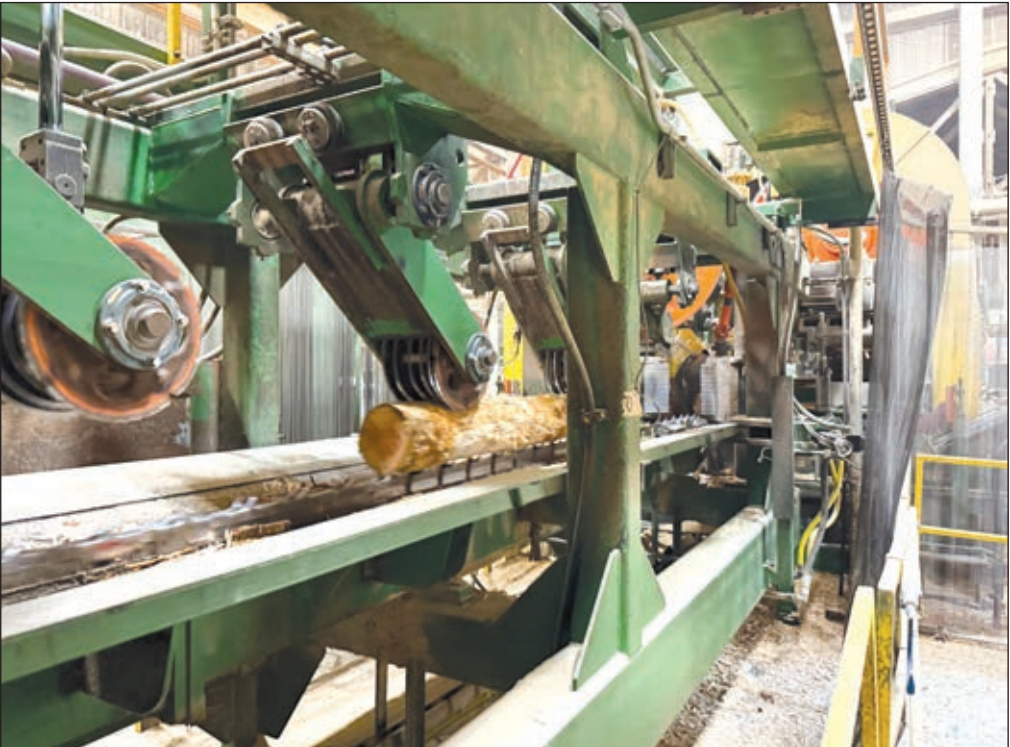
Bark is removed from logs and used in the kiln-drying process.
