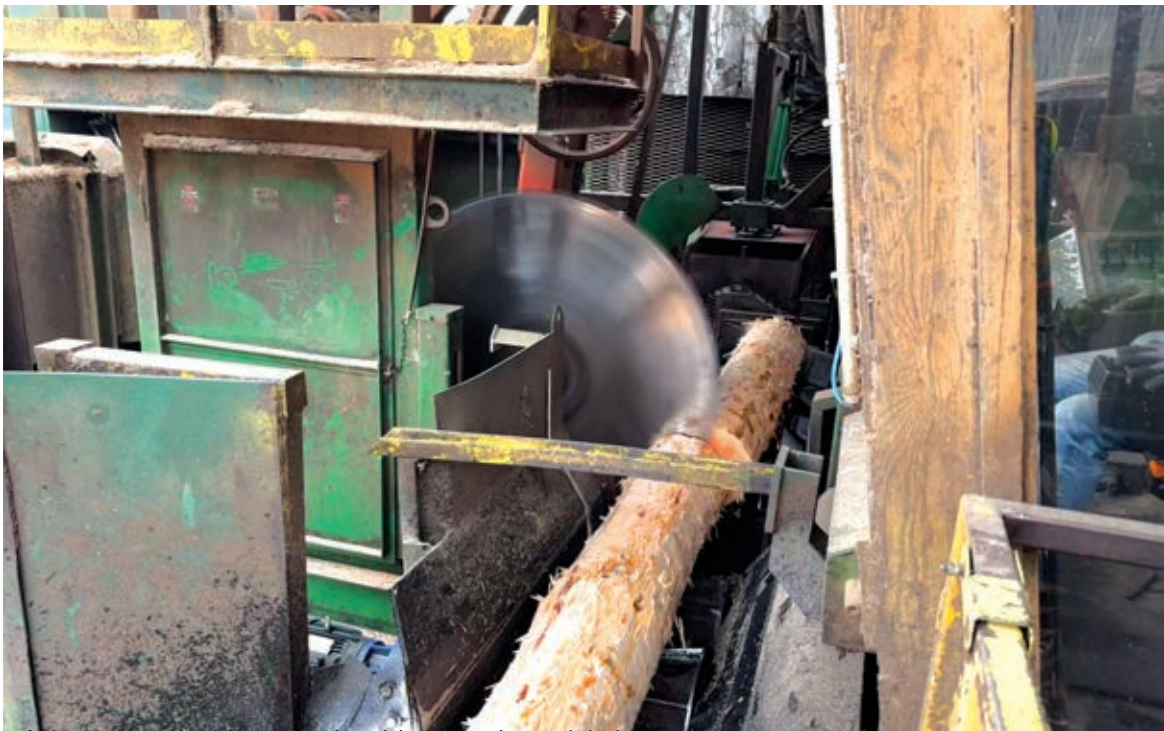
A chop saw cuts the debarked logs into eight-foot sections early in the milling process.
