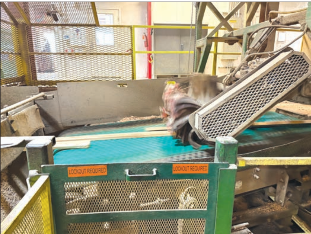
The planar smooths dried lumber to prepare it for retail.
