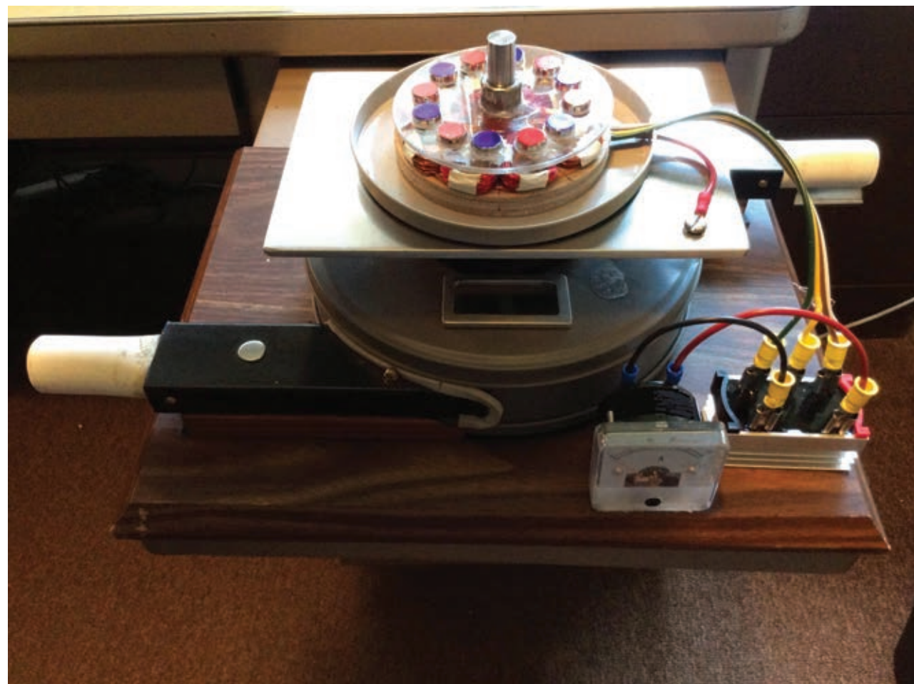
Hannah Device: The prototype for the original Hanna Turbine in WAVE configuration on display at Oregon State University's Hatfield Marine Science Visitor Center in Newport, Ore.
