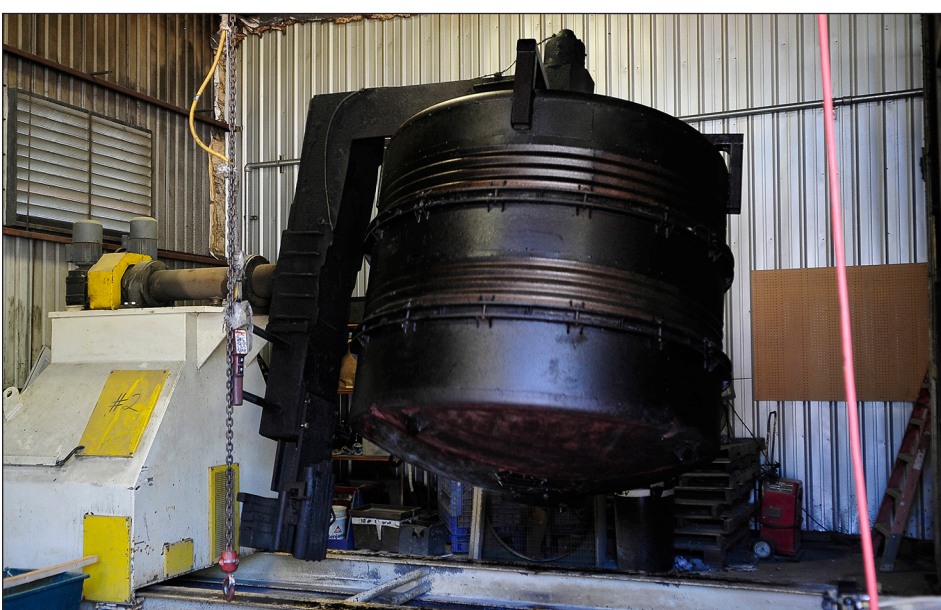
A huge form rotates as it creates a water tank at Quadel Industries.
