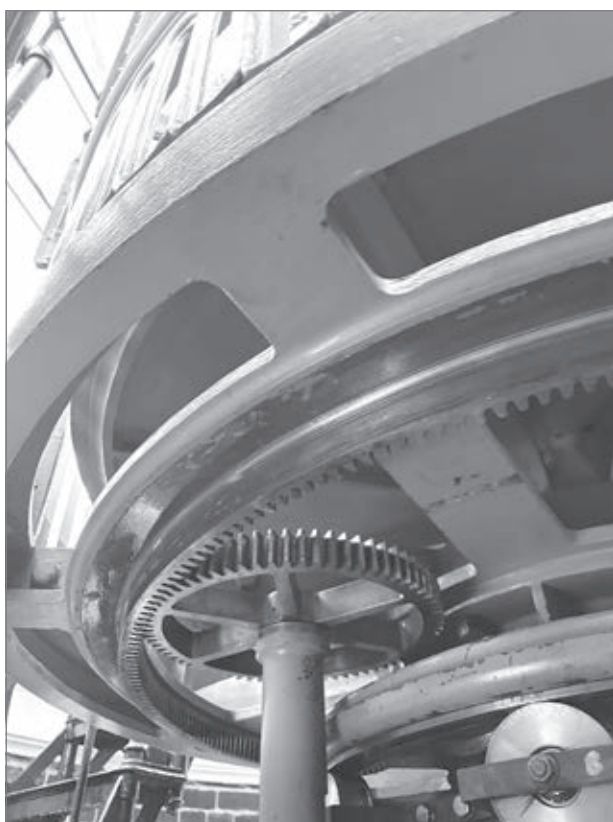
Left, the entire lens and platform inside the lighthouse is rotated by gears. Right, in the bottom right, of the photo, one of the worn carriage wheels is visible, marked with an “8.”
