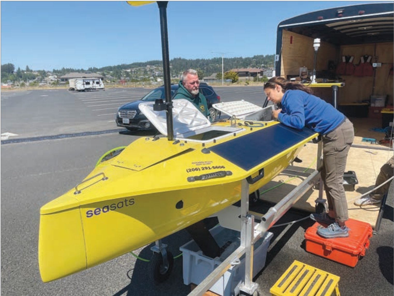
Anthony Odell, a shellfish monitoring technician with the University of Washington, and Anna Bolm, a faculty researcher at the Hatfield Marine Science Center, work on an autonomous watercraft known as a Lightfish, which gathers ocean water samples to test for biotoxins. (Photo by Steve Card)
