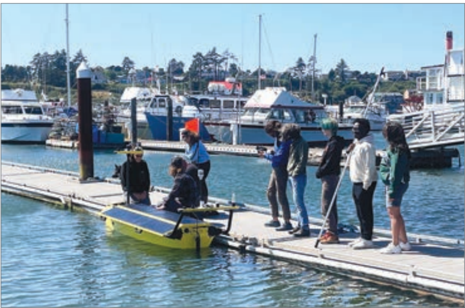
A final check is made before sending the Lightfish out of Yaquina Bay to collect water samples over a two-day period.
