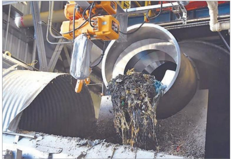
**Georgia-Pacific’s copyrighted Juno technology extracts paper fibers from mixed recyclable material for use in containerboard manufacturing, while extracting other recyclable material that can be processed at other sites. (File photo)**
