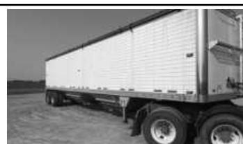
2009 Timpte Aluminum Grain Trailer/VIN# 1TDH422219B119663 40 Ft. 96" Wide, 78" High ; Spring Ride Suspension ; Tandem Axle ; Standard Hoppers ; Traps re-done 2 years ago ; Tarp new 1 year ago ; 8 Aluminum Rims ; 11R22.5 Tires - 75% ; Brakes - 50% Corrosion in King Pin and Front Rail Section ; Repairs needed on main suspension beams.
