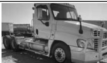
2009 Freightliner Cascadia Day Cab Truck (VIN# 1FUJGECVX9LAH0516) ; Mercedes MBE 4000 Engine - 450 HP ; Eaton Fuller 10 Speed transmission ; Air Ride suspension ; Jake Brake ; 3.42 Gear Ratio ; 180" WB ; 10 Aluminum Rims 11R22.5 Tires ; 700,000 Miles.
