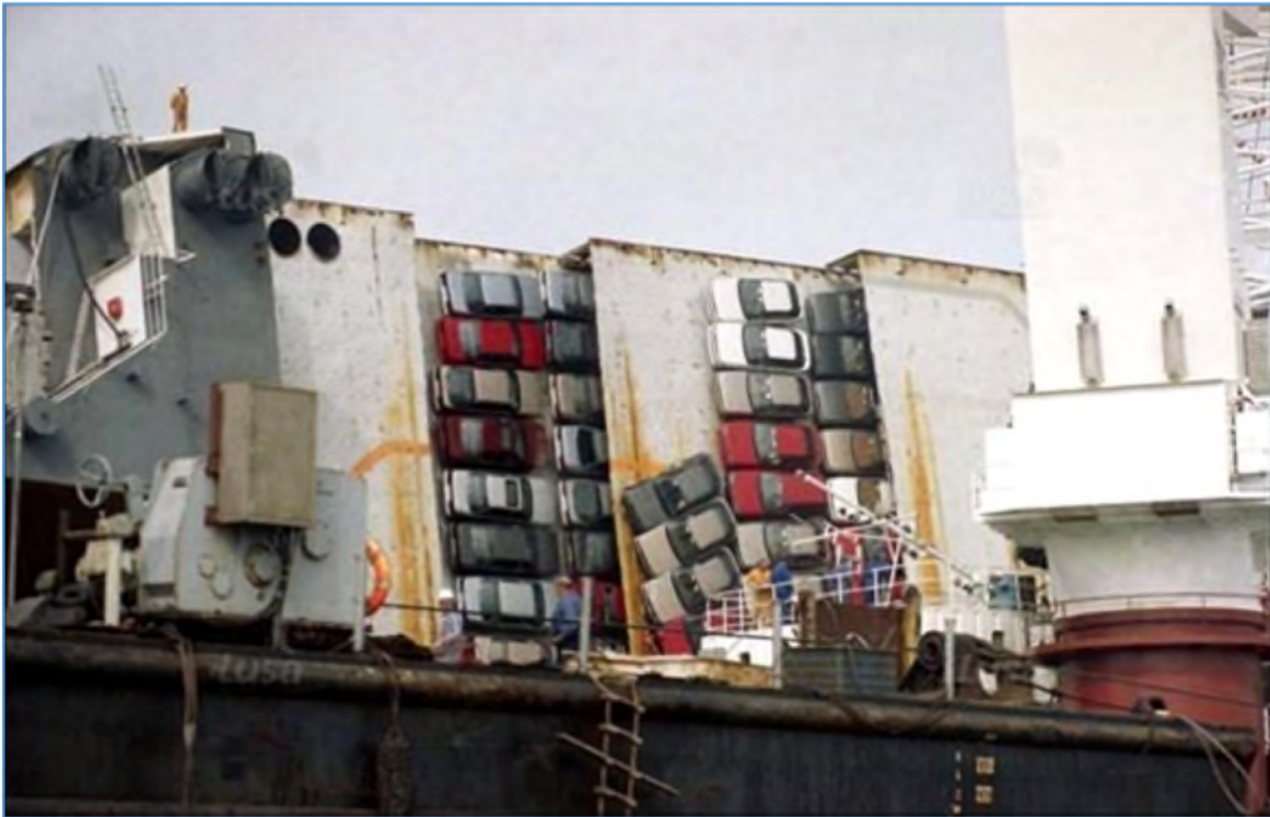
Figure 4 Photo from REIJIN salvage in Portugal showing decks being cut away and cars accessible for removal
