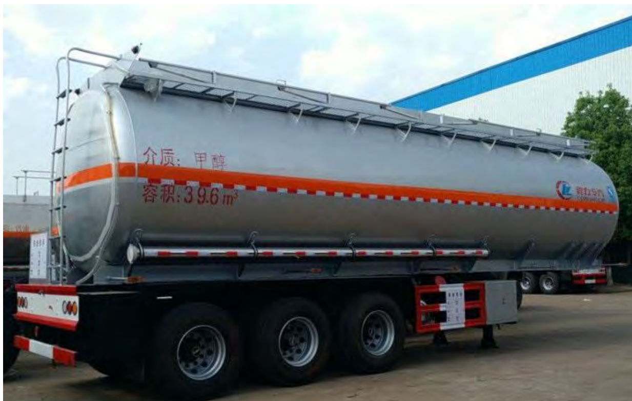
Figure 2.13. Trailer for hauling methanol in China, 39.6 m 3 capacity.
