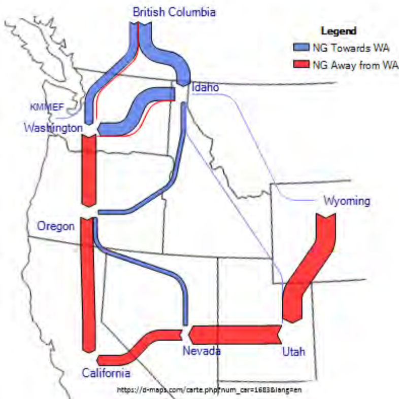
Figure 2.8. Natural gas flow.
