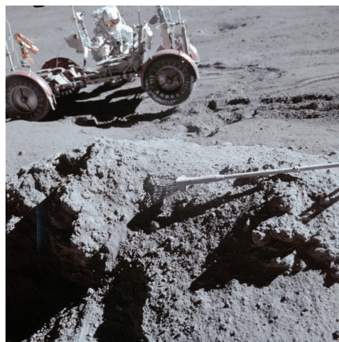
Lunar Roving Vehicle at Station 6a; note the slope is steep enough that one of the wheels is off the ground.
