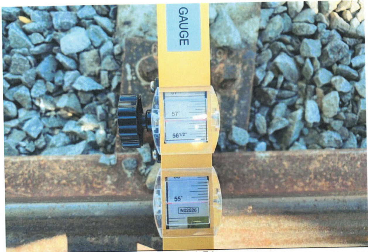
Gauge for Curve in Tolerance
