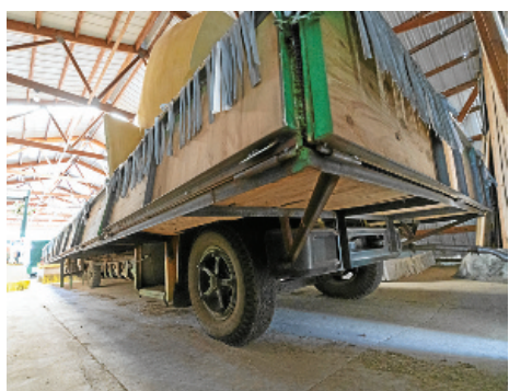
The De Klompen float is built backwards on the chassis of a bus with the steering wheel in back.
