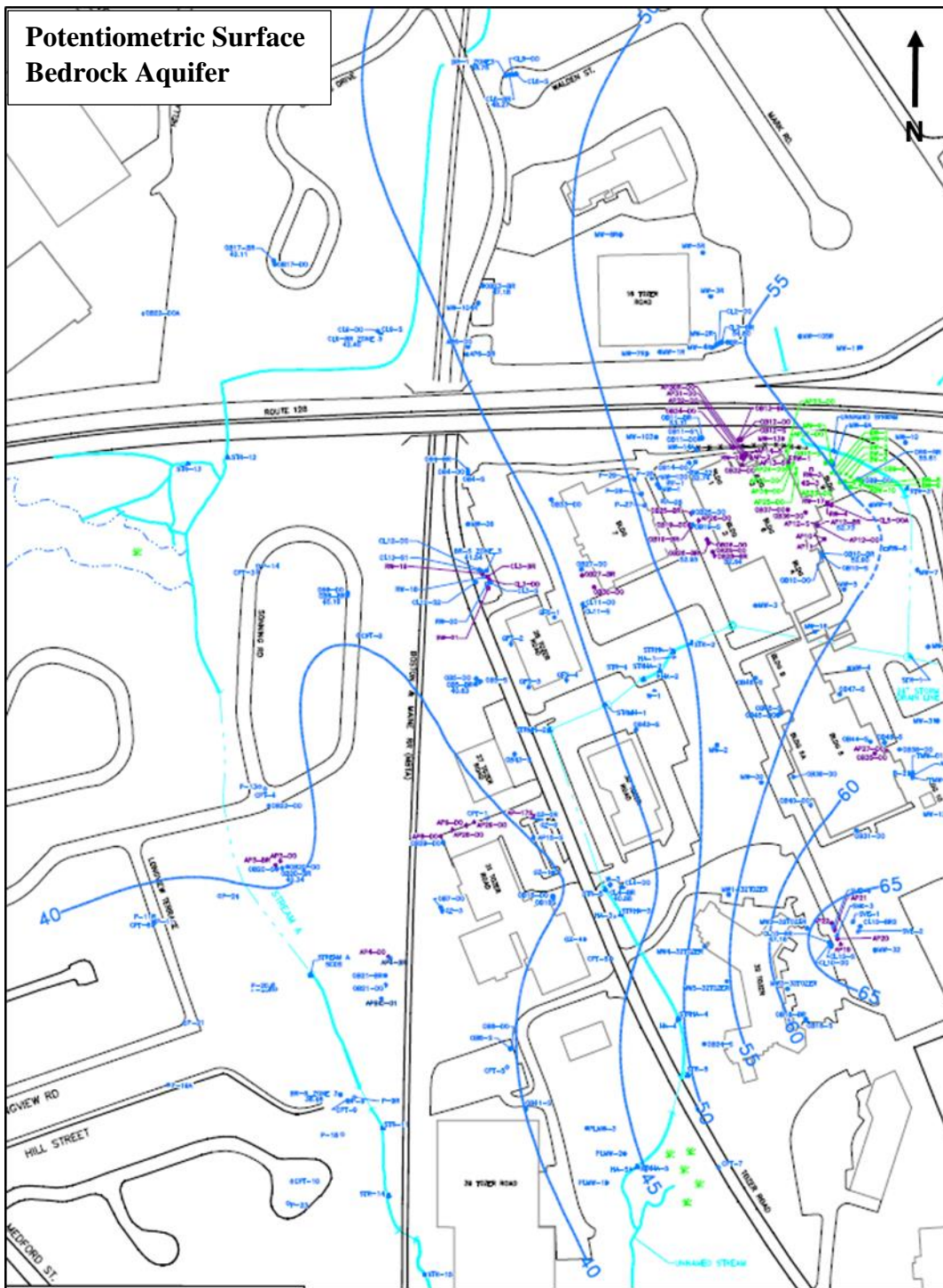
Figure 5. Potentiometric surface map of the bedrock aquifer shows groundwater flowing west from the former Varian facility.
