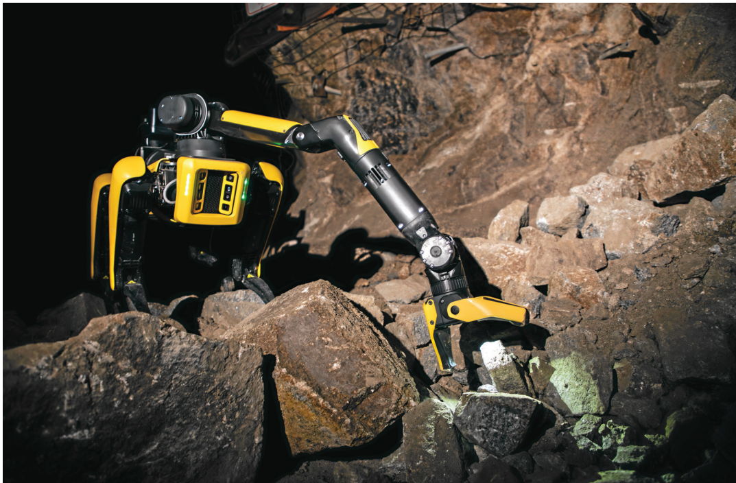
SPOT, a four-legged robot about the size of a large dog, reaches to grab a rock in the Underground Mine Education Center at Montana Tech. Mining Engineering Associate Professor Abhishek Choudhury and a group of students have been working with SPOT to see if the robot can travel through abandoned mines which might be unsafe for humans and gather samples in the search for critical minerals.
