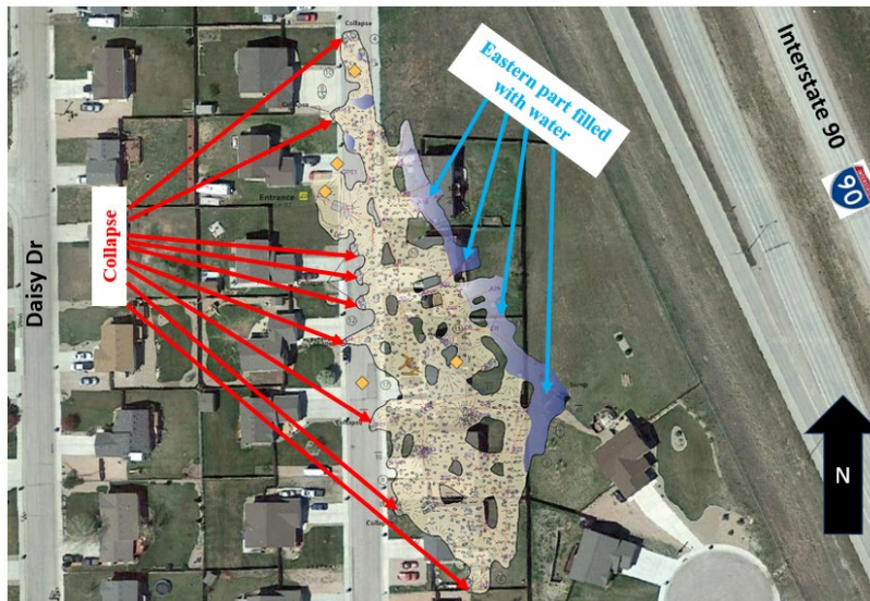
Figure 2. Approximate extent of the underground mine developed by Paha Sapa Grotto cavers (Wolfe et al. 2020) overlaid on the subdivision by Patrick Ealy, Fitzgerald Law Firm (Zionts 2020)
