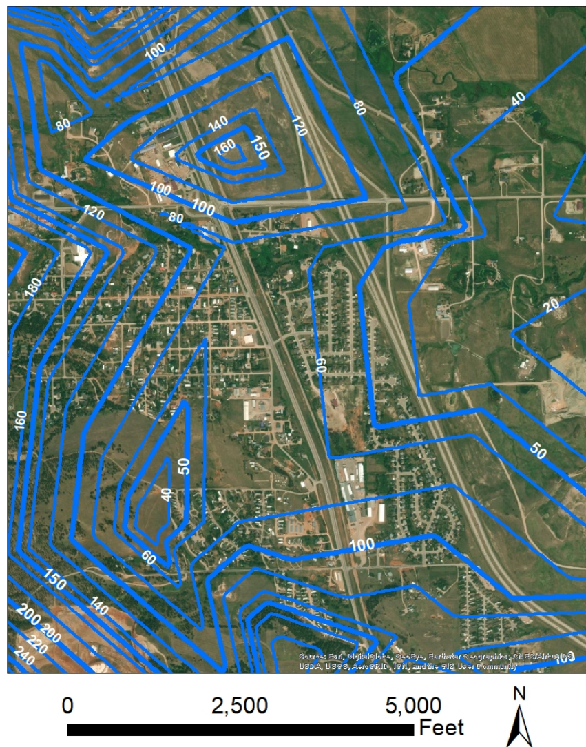
Figure 5. Contours of the depth to the groundwater table (in ft.) in the area
