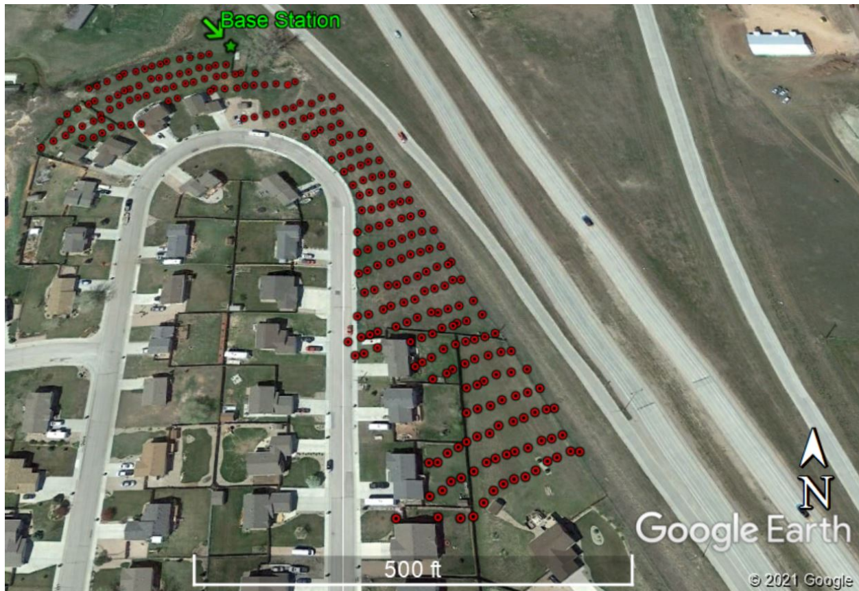
Figure 7. Locations of the base station and variable points used in the SP measurements
