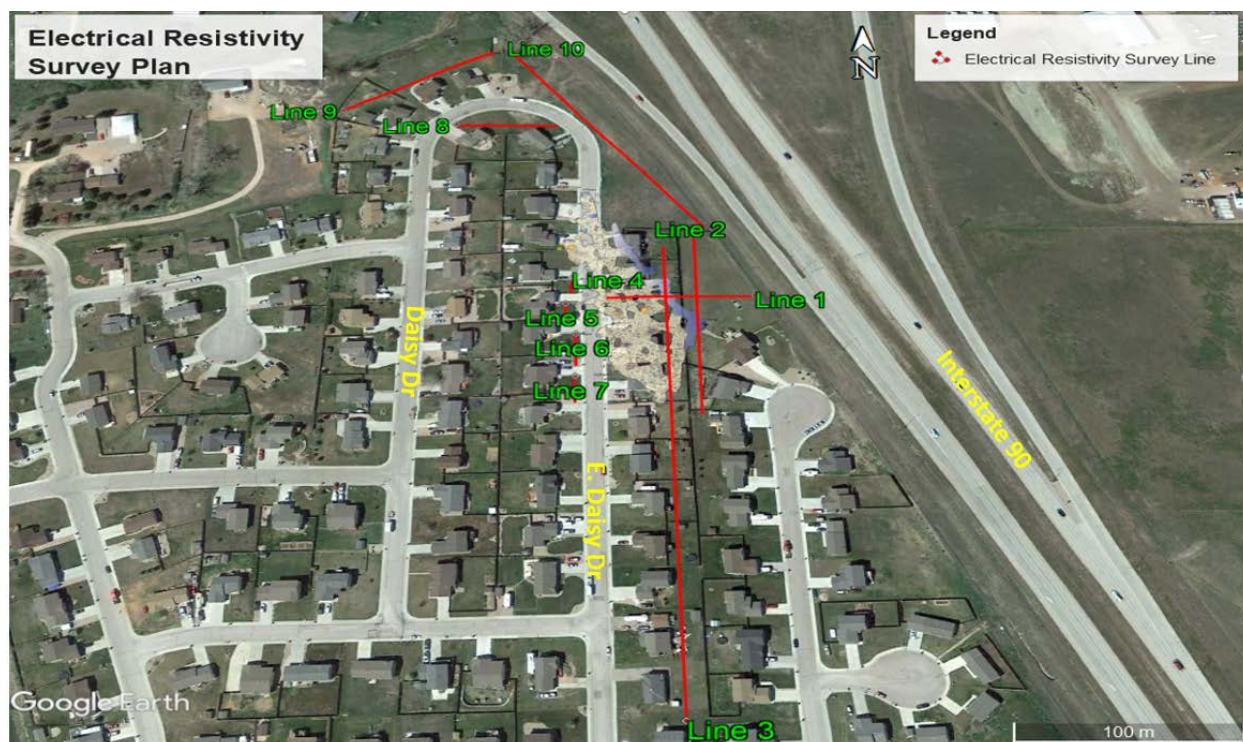
Figure 7. Proposed Electrical Resistivity Tomography survey lines
