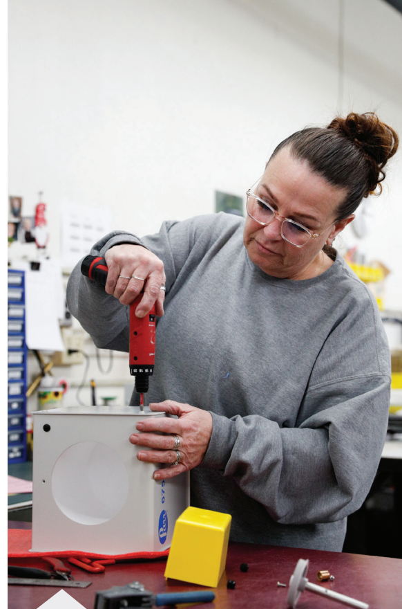
A worker assembles a component to a Parr 6755 Solution Calorimeter at Parr Instruments.
