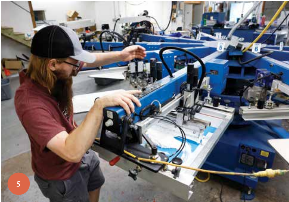
5. Mike Johnson test prints a t-shirt on a screen printing press at QC Custom Tees & More. An automatic squeegee is used to pass the ink over the screen. 6. Sean Rupp shows off a freshly made screen after emulsion is washed off. Katelyn Metzger
