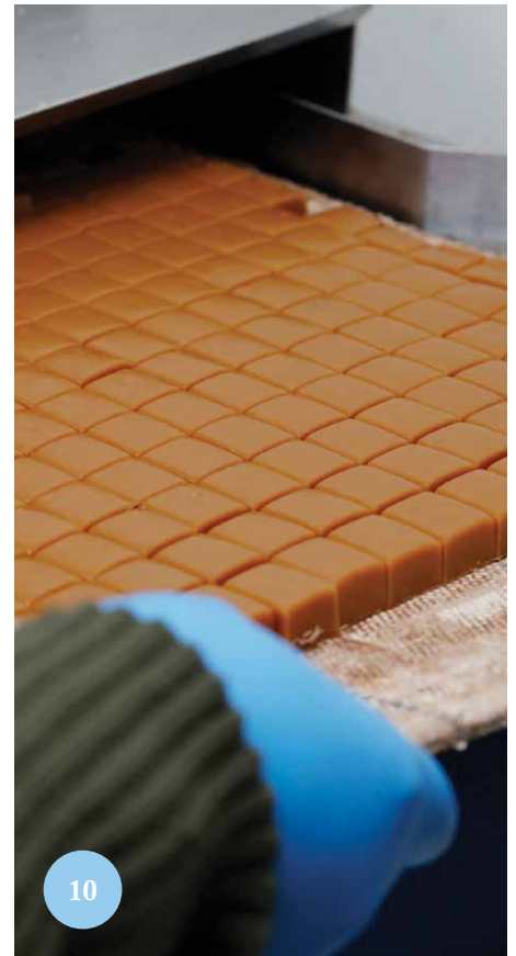
5. Daniel Otten places pecan dainties onto the enrober belt, which will cover the candies in tempered chocolate. 6. Lagomarcino's manager Daniel Otten shows off the enrober, which melts and tempers up to 400 pounds of chocolate at once, on Thursday, Feb. 5, in Davenport. 7. The enrober melts and tempers large amounts of chocolate, keeping it at about 83 degrees, which gives the chocolate a shiny sheen. 8. Daniel Otten picks up freshly made pecan dainties off of the conveyor belt on Thursday, Feb. 5, in Davenport. It takes about 15 minutes for chocolates to get through the cooling portion of the enrobing machine. 9. An old Lagomarcino's metal sign hangs in the Village of East Davenport on Thursday, Feb. 5, in Davenport. 10. Daniel Otten cuts a tray of caramels at Lagomarcino's on Thursday, Feb. 5, in Davenport.
