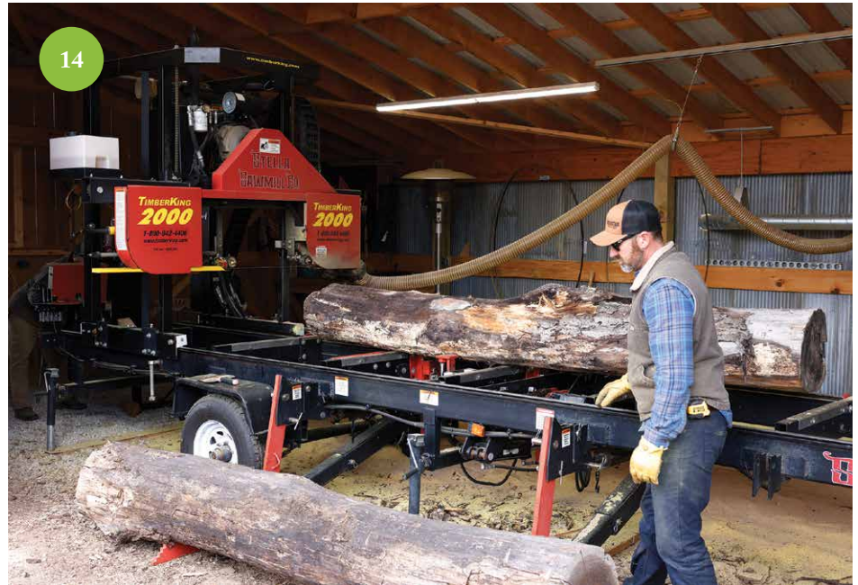
13. A look at Stella Sawmill's vacuum kiln on Thursday, Nov. 6, in Milan. 14. Nick DeVolder looks over a log ready to be cut at Stella Sawmill on Thursday, Nov. 6, in Milan. Because trees rest before they are milled, the end grain of the logs are sealed with a wax-like substance to reduce cracking.
