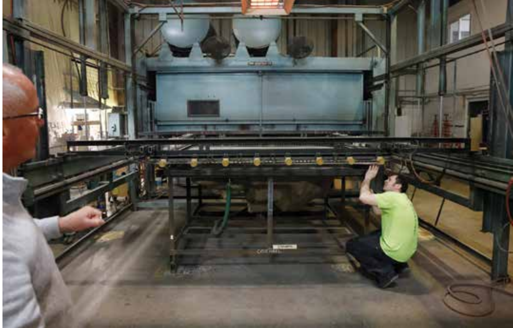
(Above) A sheet of acrylic is cleaned and heated before being molded into a hot tub. (Right) Jim Kettleson shows off the different sheets of acrylic that will be later molded into a hot tub or spa.
