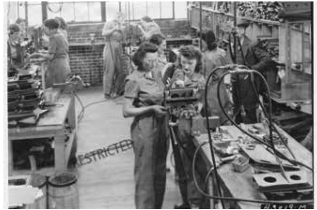
Women complete drilling, riveting and assembly into sub-assemblies for the Grumman T.B.F. Avenger torpedo destroyer at John Deere Harvester Works in 1943. Courtesy of John Deere
