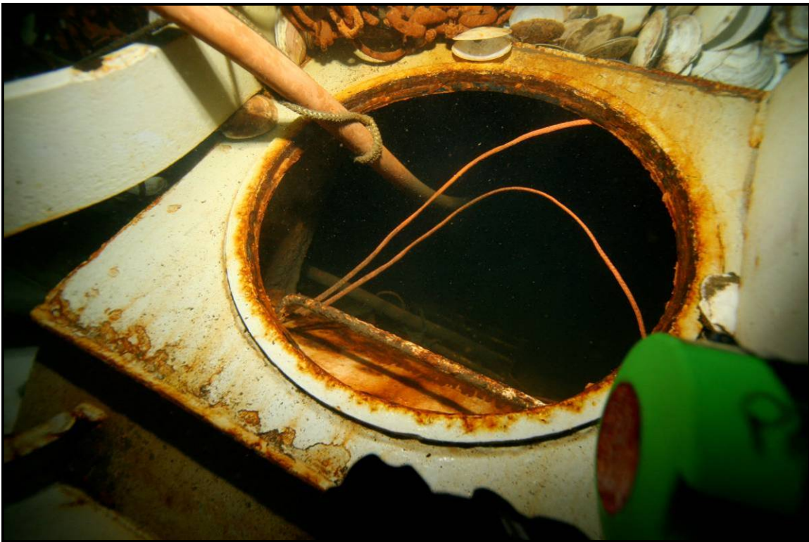
Figure 14: Open lazarette access point located just forward of the transom, port side.
