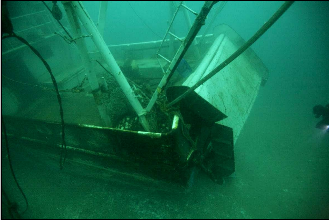
Figure 18: The damaged stern ramp
