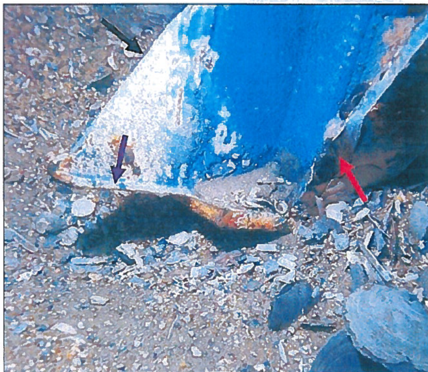
Figure 19. The structure at the rear of the vessel where the skeg is normally attached.
