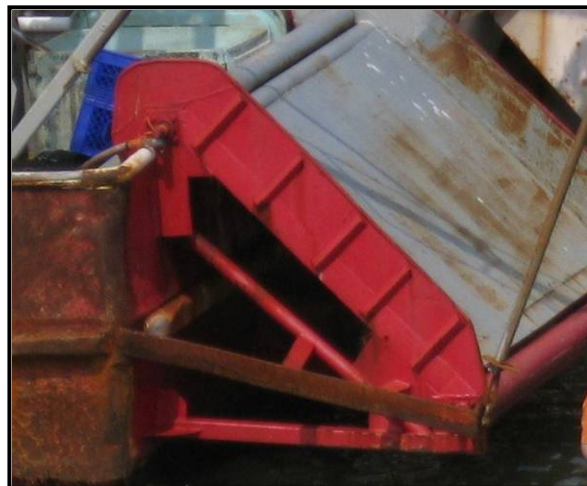
Figure 24: Stern ramp showing flat bar
