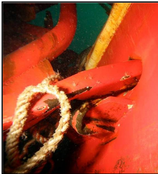
Figure 20: View looking up from under the ramp to the punctured transom
