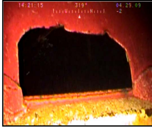
Figure 12: Starboard aft freeing port
