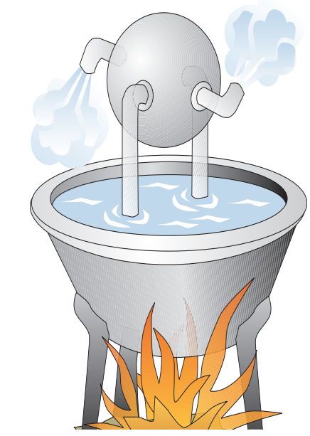
Early Greek engine, A.D. 62 Thrust from exhausted steam caused the sphere to rotate.
