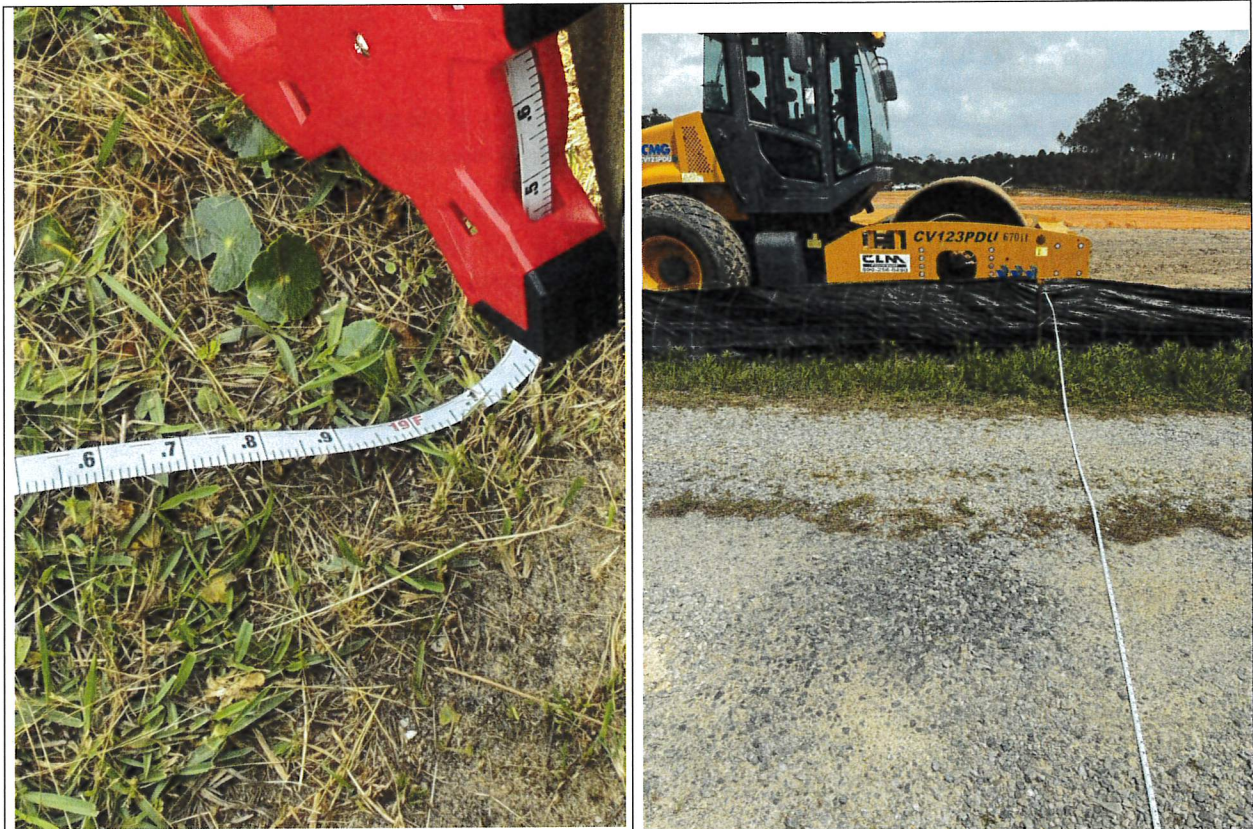
Photos 1 and 2: Measurement of distance from silt fence to western edge of Madison Place | 25 ft. ingress and egress and drainage easement is approximately 19 ft. This distance including appropriate buffering should exceed 25 ft.
