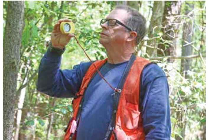
Dean uses a clinometer to measure tree height using the principle of measurement called triangulation.
