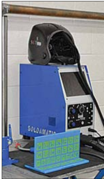
A virtual welder gives beginning welding students at SCC practice before moving to authentic welding.
