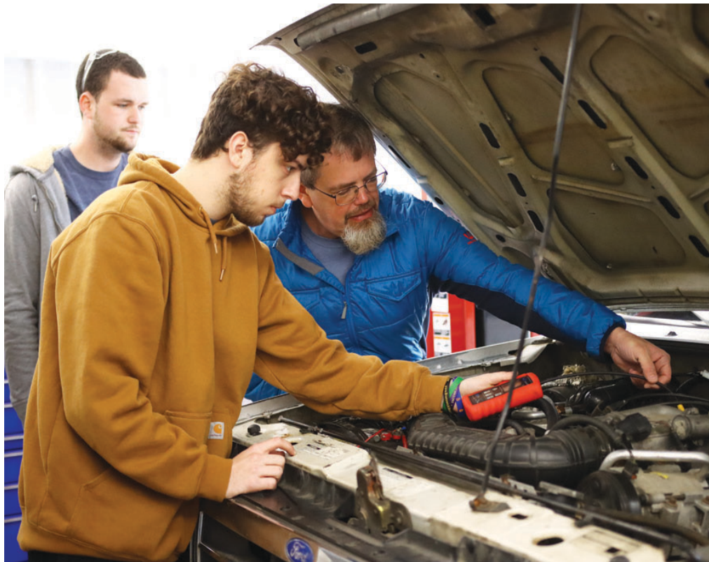
Southeastern Community College students learn to use an ignition tester during engine performance lab with instructor Johnny O'Connell.
