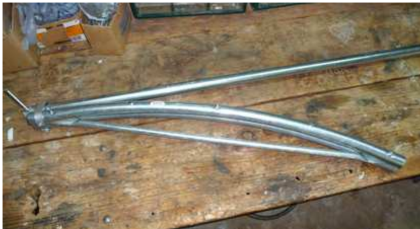
A 'Quick Hoops' tube bender mounted to a shop bench. For more information on this bender, go to Shop Hoop Benders .
