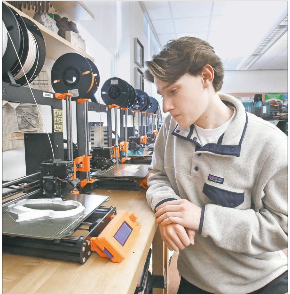
Senior Graydon Conly watches as the plastic body of his penguin-shaped induction flashlight is made from his specifications by a 3D printer in March.
