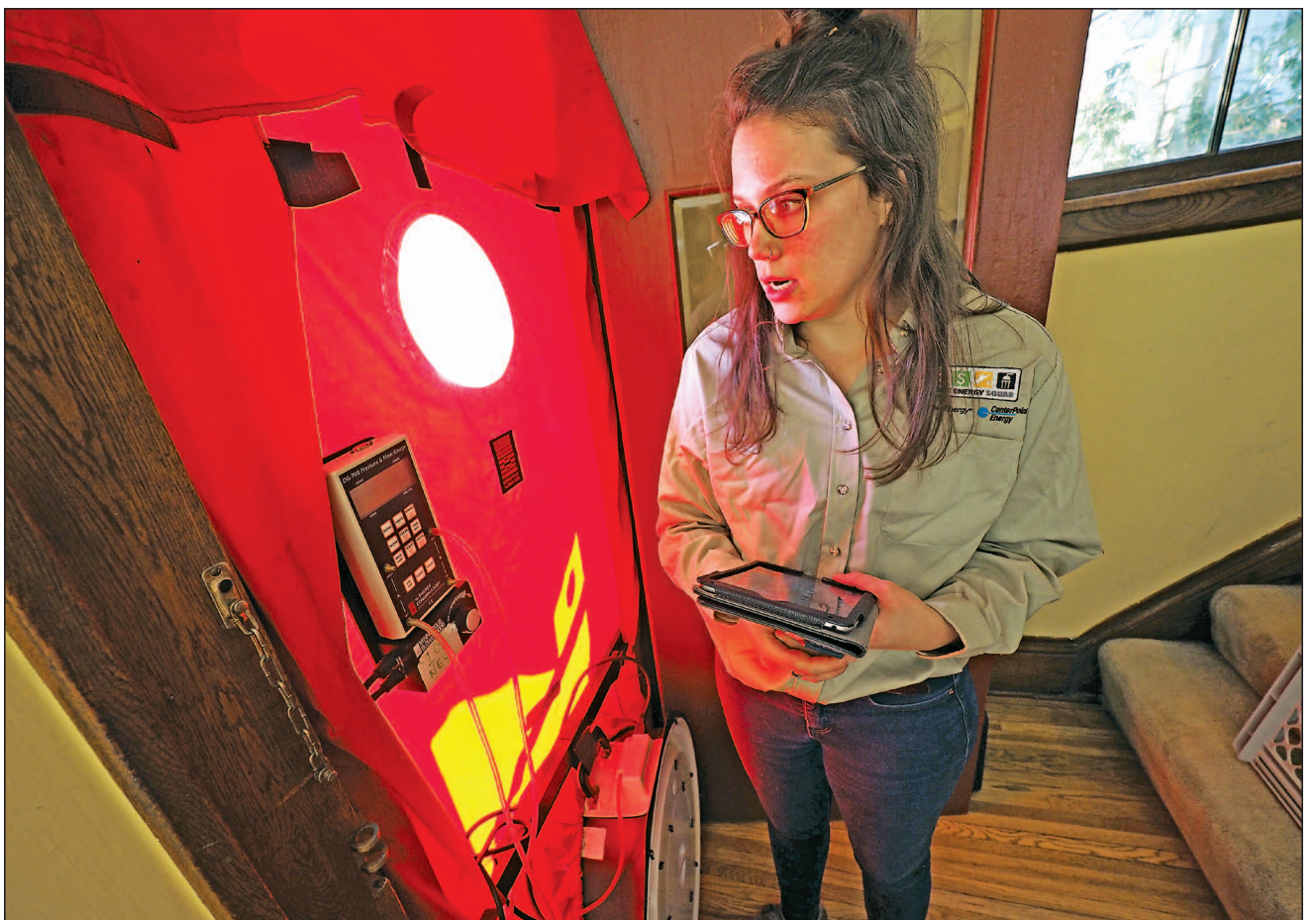
Home Energy Squad energy auditor Kristin Syverud conducts a blower door test at a Highland Park home to check for air leaks. PHOTOS BY BRAD STAUFFER
