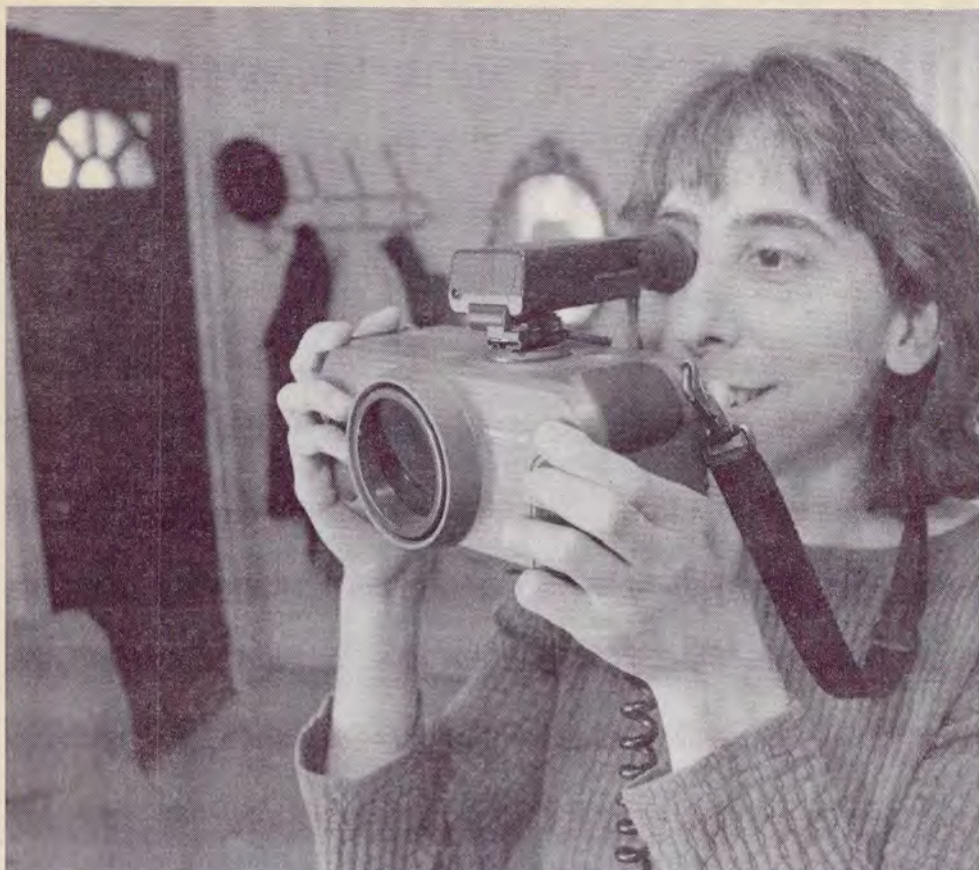
Diana Cohen, contract coordinator for the St. Paul Neighborhood Energy Consortium, uses an infrared scanner to check the insulation in the wall of a Macalester-Groveland home. Photo by Kristine Heykants.
