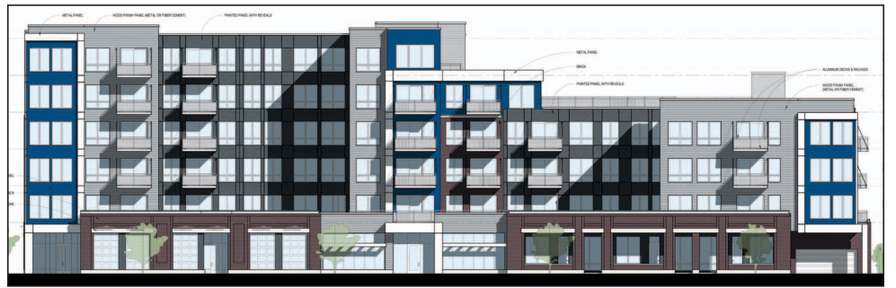
TJL Development's latest plan for a 118-unit market rate apartment building with first floor retail on the southeast corner of Snelling and St. Clair avenues features a stepped-back design and heights of from 47 feet to 68 feet 4 inches.
