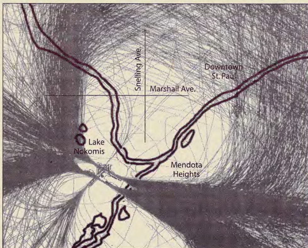
This diagram shows the flight paths of the 2,948 airplanes taking off from the three runways at Minneapolis-St. Paul International Airport during one week in June 1997.
