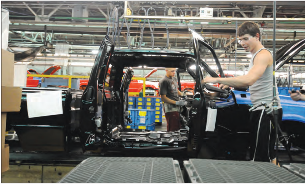
The Highland plant currently employs 968 workers, shown installing window trim (above) and attaching the nameplate on a new Ranger (right). PHOTOS BY ANNE BRANDRUD
