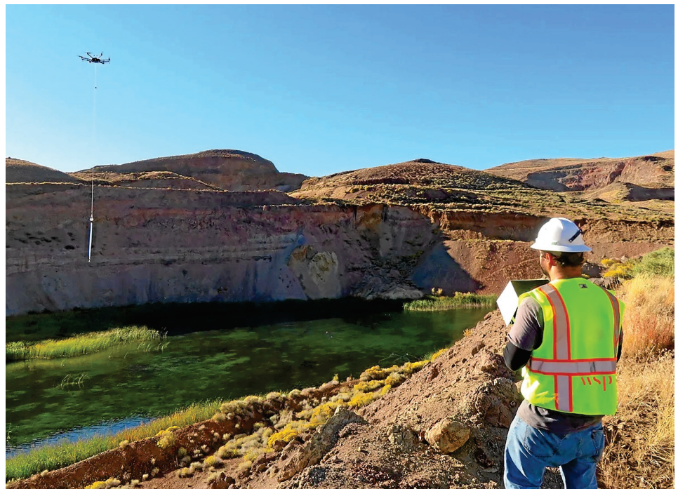
WSP engineers use drones to collect pit lake water samples.
