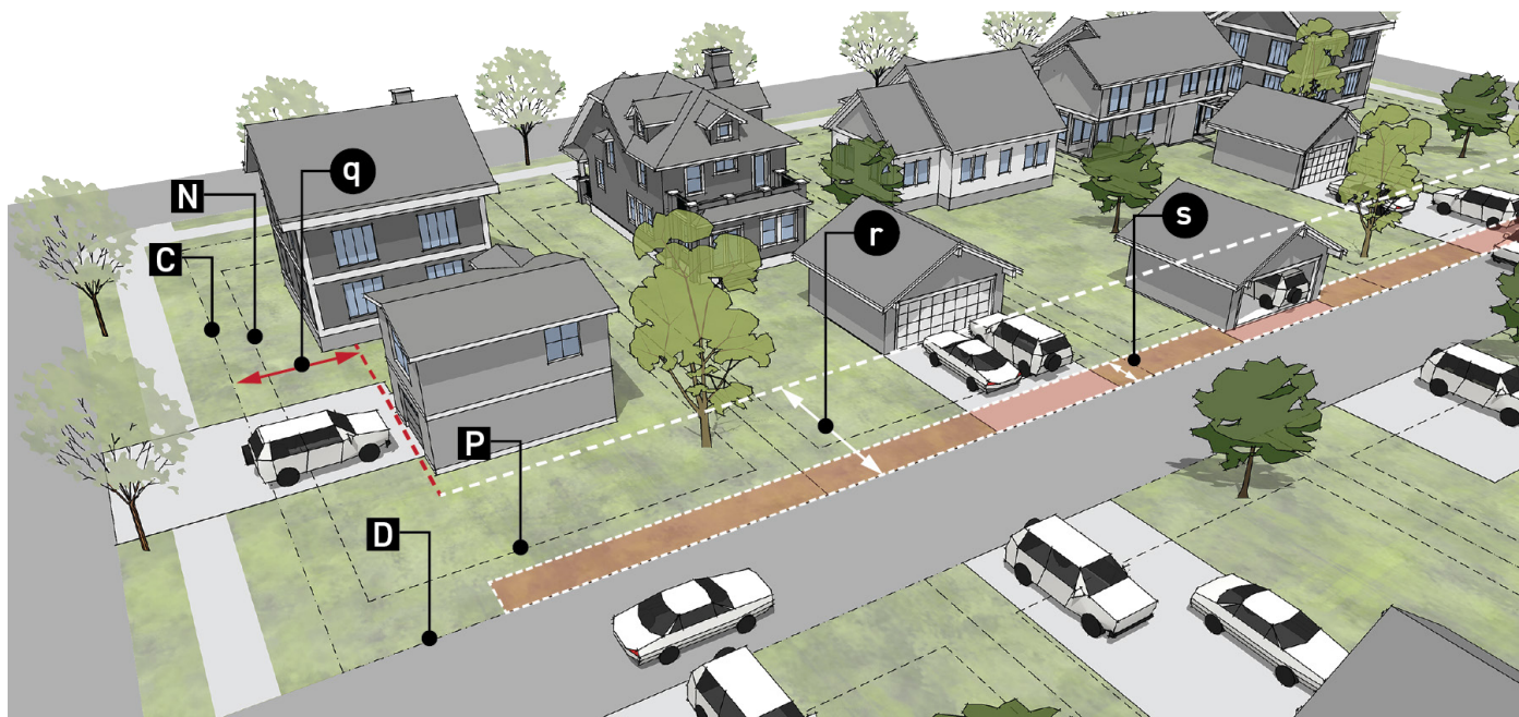
FIG. 15 Alley and Side Access Setbacks
