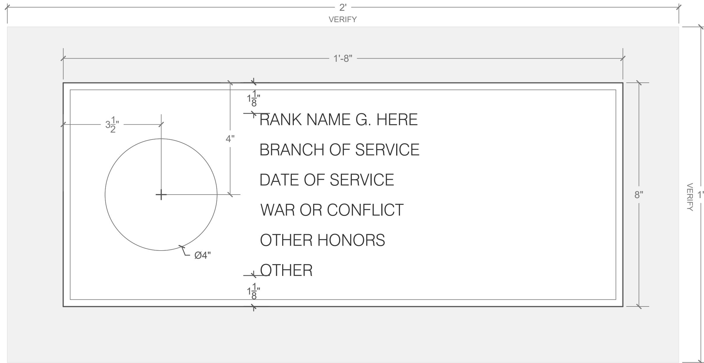
PLAQUE SIZE ON BLOCK ELEVATION - SCALE: 6" = 1'-0"
