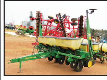
USED John Deere 7200 Corn Planter , 4 row narrow, no-til, dry fertilizer, finger, double disc openers, press wheels, closing wheels, insecticide boxes, markers, 7.60-15 tires #H28530..... $7,500
