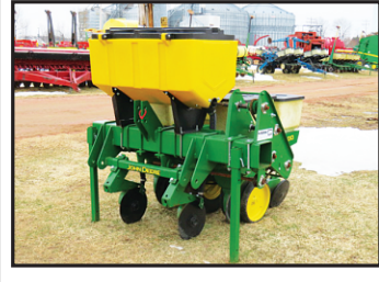
USED John Deere 7100 Corn Planter , 2 row narrow, dry fertilizer, 3pt hook up, ground drive, insecticide boxes, press wheels, closing wheels, 7.50-16 tires #H28528..... $4,400
