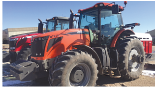
2009 AGCO DT275B CVT - 32 MPH - FULL WT. PACKAGE - 710X42 REARS FRONT & REAR DUALS - 5 REMOTES - 3800 HRS.
