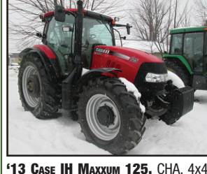
'13 CASE IH MAXXUM 125 , CHA, 4x4, 540/1,000 PTO, 2 Hyd. Remotes, 10 Front Wts., 16x16 PS, 125 HP, 870 Hrs., #C19409 ..... $69,995
