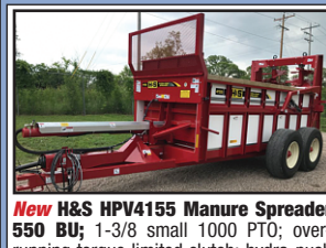
New H&S HPV4155 Manure Spreader 550 BU; 1-3/8 small 1000 PTO; over-running torque limited clutch; hydra-push manure spreader w/vertical beaters; Tires: 425 x 22.5. E40119 . . . . $8,966
