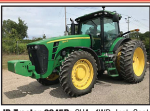
JD Tractor 8245R; CHA, 4WD, Inst. Seat, Diff Lock, CD Player, 16F/4R P.S. Trans, 540/1000 PTO, 3 Pt, Top Link, Qck Hitch, 4 Rmts, 20 Ft Weights, Beacon, Blk Htr, 6 Cyl Turbo, 245HP, Frt Fenders, 480/80R50 W/Duals. EX0565 . . . . $119,999
