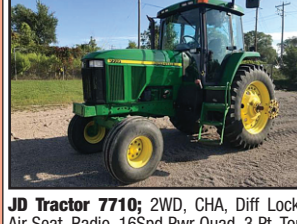
JD Tractor 7710; 2WD, CHA, Diff Lock, Air Seat, Radio, 16Spd Pwr Quad, 3 Pt, Top Link, 3 Rmts, 540/1000PTO, 6 Cyl, 155Hp, 18.4R42 W/Duals. Super Clean! E40597 . . . . $47,770
