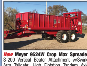
New Meyer 9524W Crop Max Spreader S-200 Vertical Beater Attachment w/Swing Arm Tailgate; High Flotation Tandem Axle Trailer w/30000lb Spring Axles; Slider System; Hydraulic Controlled Brakes; 710/50x26.5 18 Ply Heavy Duty Radial Flotation Tires Mounted on 26.5x24 Wheels. E39629 . . . . $75,999
