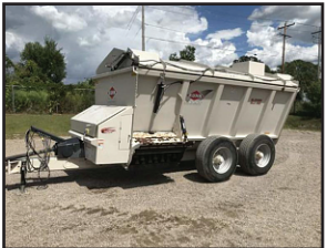
Kuhn/Knight Spreader SLC132; Side Slinger Spreader, Protwin, Hydraulic lid, Small 1000 PTO, 3200 Gal, 385/65R22.5 Tires. EX0536 . . . . . $39,500
