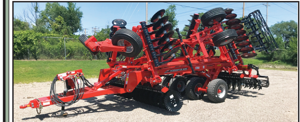
Kuhn Krause Tillage IntercePTOR 8050-20; Aggressive High Speed Tillage, 54 Blades, 9" Spacing, 19' Working Width 20' Cut Width, 22" Diameter 32 Flute Excalibur Ct Shallow Concavity Blades, Aprox 18,407Lbs. E39060. . . . $72,999
