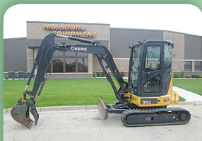
2015 Deere 35G Compact Excavator 383 Hrs, 23.3 HP, Yanmar Engine, Dig Depth- 10 Ft, Dig Height- 11 Ft 4in, Transport Length- 15Ft 3in, Cab A/C, Radio, Long Arm, 12" Pads, 12" Bucket
