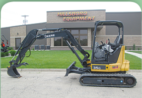
2015 Deere 35G Compact Excavator 539 Hrs, 23.3 HP, Yanmar Engine, Dig Depth- 10 Ft, Dig Height- 11 Ft 4in, Transport Length- 15Ft 3 In, ROPS, Long Arm, 12" Pads.
