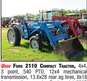
USED FORD 2110 COMPACT TRACTOR , 4x4, 3 point, 540 PTO, 12x4 mechanical transmission, 13.6x28 rear ag tires, 6x18 front ag tires, used - Ford model 776B quick attach loader with joystick, pin on 66" bucket ..... $12,500
