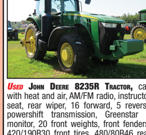
USED JOHN DEERE 8235R TRACTOR , cab with heat and air, AM/FM radio, instructor seat, rear wiper, 16 forward, 5 reverse powershift transmission, Greenstar 3 monitor, 20 front weights, front fenders, 420/190R30 front tires, 480/80R46 rear tires with hubs and mounted duals, 4 remotes, 3 point, quick hitch, 1 3/4" 1000 PTO ..... $97,500
