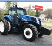
sed NH T8.320 Tractor; deluxe cab; electric mirrors; front HID & LED ork lights; single beacon; NAV II w/372 Rec Waas; large color monitor; block heater; high cap drawbar; high cap hyds; 6 sets remotes; power peyond return; 540/1000 pto; 480/90R50 RT w/ axle duals; 420/85R34 Trelleborg FT; front fenders; 12-88 lbfrt weights; front axle susp; hyd trailer
