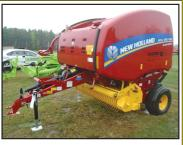
ew New Holland 450 Roll-Belt Round Baler: silage version 4x5 bale size, net and twine, 540 RPM PTO, 31x13.5-15 8 PR tires, 1.8M pickup, 15x6.00 caster wheels, manual hydraulic pick lift windgauard roller ISO control with monitor A48780
