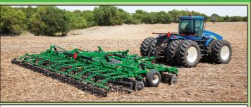
Great Plains 1200TM Turbo Max; Vertical Tillage Disc, 12' Wide, 20"x256" Turbo Blades @ 7.5" Spacing, Extra HD C-Shanks, Wing Flex of 10", Walking Tandems on Center Transport, Dual Wing Tires, Constant Level Hitch Single Tongue Case Hitch, Single Point Depth Adjustment, Rolling Harrow & HD Reel, Safety Lights..
