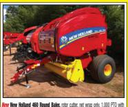
cut out clutch, makes a 4' x 6' bales, 15 x 6.00 - 6 castering pickup wheels, drawbar hitch, manual hydraulic pick up lift, endless belt, manual rotor reverse, 5 bar pick up reel with assist, 2.07m pickup assist, moisture sensor, 21.5L x 16.1 10 PR tires, A50524
