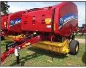
nd RB450 Round Baler Roll-belt 450; 4x5; silage 1.8m; endless belt; deluxe wrap; net only; 540 RPM with cut-out-clutch; 31x13.5-15 8 PR wheels and tires; manual hydraulic pickup lift-ff; 5 bar pickup reel; 7.8m roller windguard. E40193
